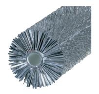
Spine Fin Coil - exclusive to Trane contains thousands of tiny fins bonded to continuous aluminum refrigerant tubing, creating greater surface area, helping with heat transfer.
